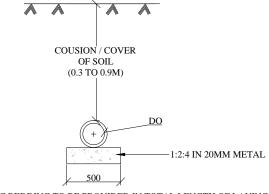
CC BEDDING TO BE PROVIDED IN TOTAL LENGTH OF LAYING OF SEWER
