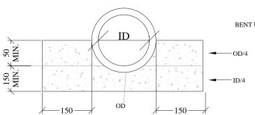
TO BE PROVIDED IN TOTAL LENGTH OF LAYING OF SEWER
